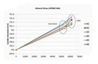
With the LDM, the same six cylinders could be measured on one working day and by one operator. The results were very similar.
