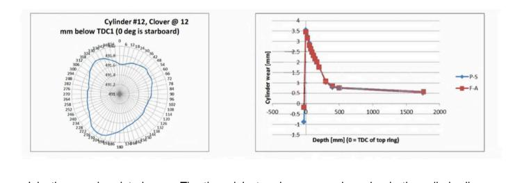
Injection nozzle related wear. The three injectors have caused erosion in the cylinder liner, turning it into a three-clover. The diameter in the P-S and F-A directions are identical so no abnormality is picked up from a wear measurement. However, the clover measurement reveals that the cylinder is in poor condition and in need of honing or replacement.
