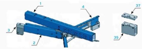
The LDM can be adjusted to suit additional bore sizes by using extra parts:
