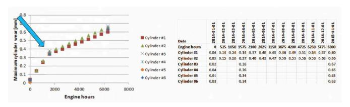
In the above example, monthly LDM measurements were done for a new engine in units #1 and #2. The wear rate was found to be too high (0.2mm / 1 000h) and the root cause was traced as cold corrosion. The counter-measures included introduction of a new lubricant and to increase the cylinder wall temperature. The result could be clearly seen as reduced cylinder wear rate.
