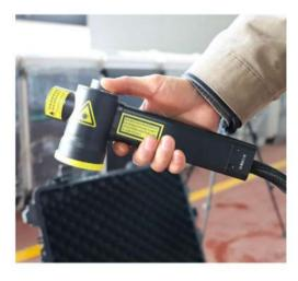
focus position under different field lenses by using the red light indicator, which solves the problems of inaccurate focus and single adjustment method of existing products on the market.
